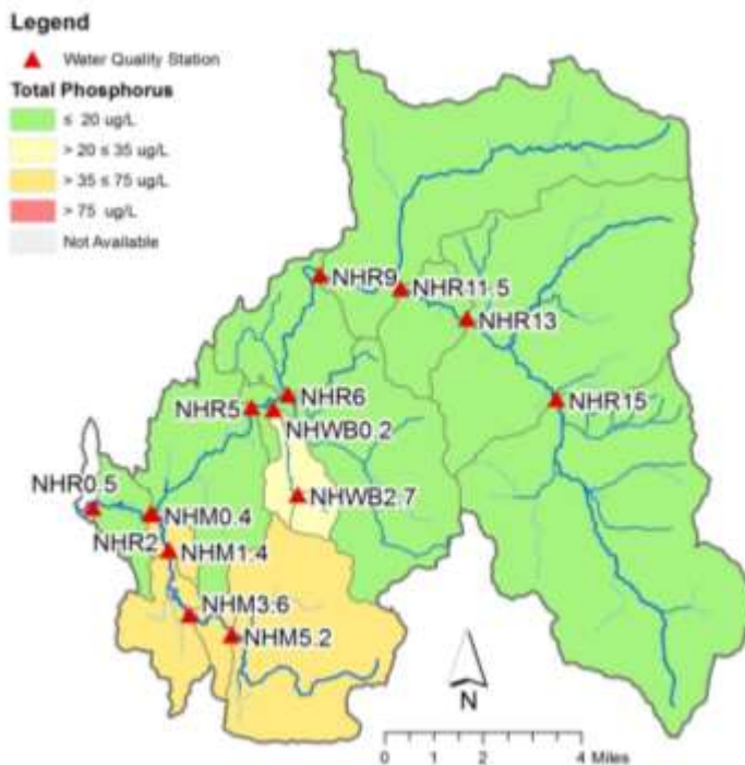
Figure 6. Mean value of Total Phosphorus detected in July, August and September (2016) during base flow conditions at or below the Low-Median-Monthly Flow in the New Haven River watershed.
