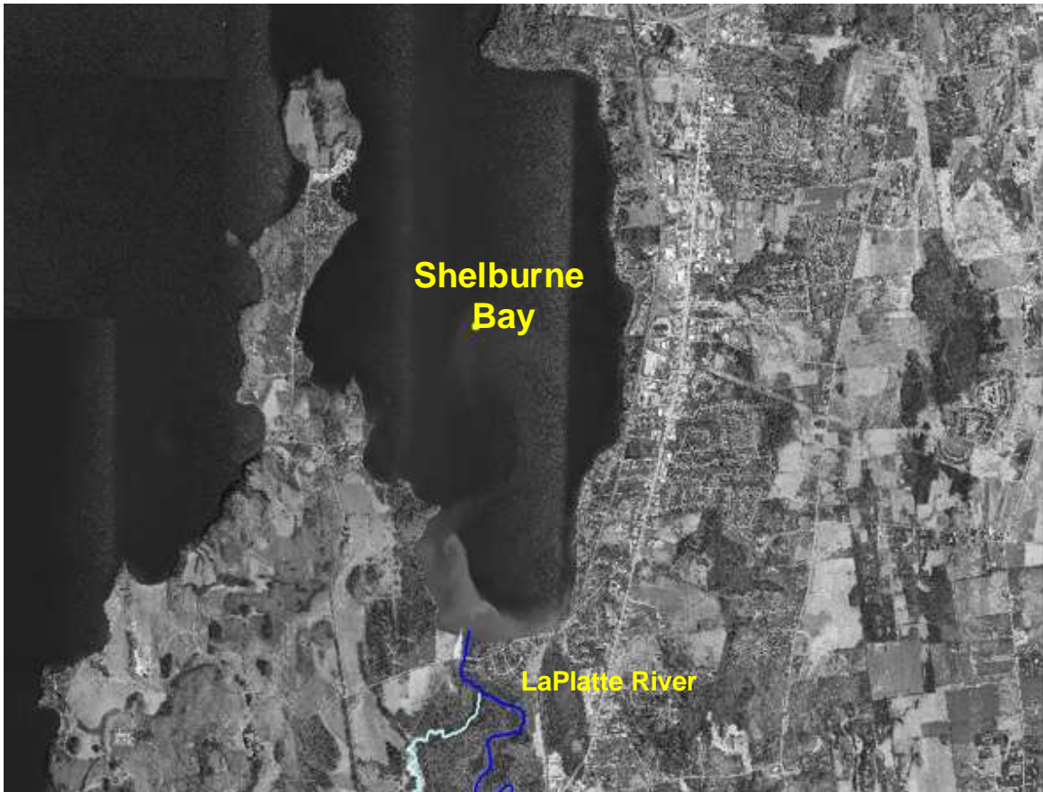
Orthophoto showing typical discharge of suspended sediment into the southern end of Shelburne Bay from the LaPlatte River during spring runoff.
