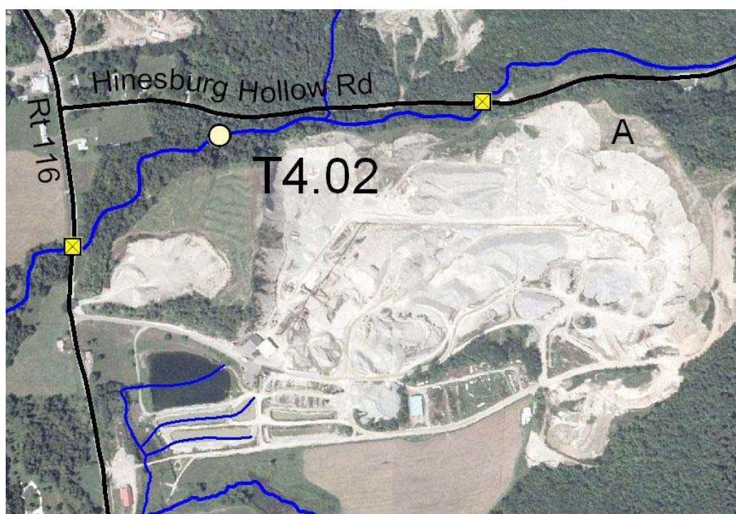
Figure 39. Potential site of Hollow Brook stream capture by Hinesburg sand & gravel quarry. (Base image: 2003. Yellow squares indicate bridge crossings with a span that is constricting to the flood-prone width of the channel.)
