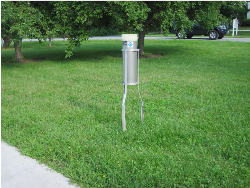
Post-Construction, July 23, 2021: NOAA rain gage.
