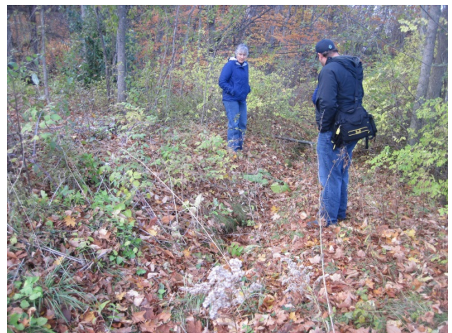
Figure 12: Gully erosion is migrating farther to the northeast along the swale (between the two people).
