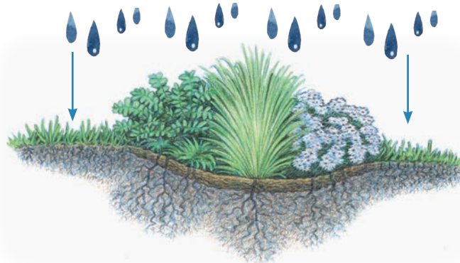
Figure 3: Stormwater that soaks into the ground close to where it falls is an important strategy for managing stormwater.
