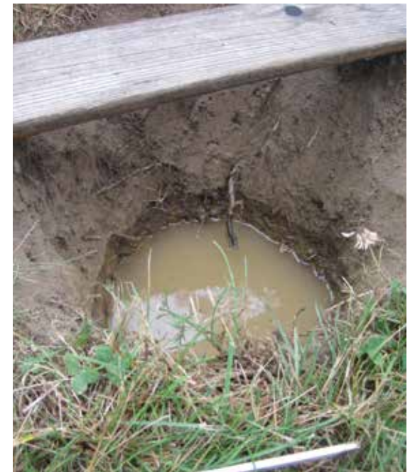
Time how long it takes for the water to drain. Repeat this to get three measurements.
