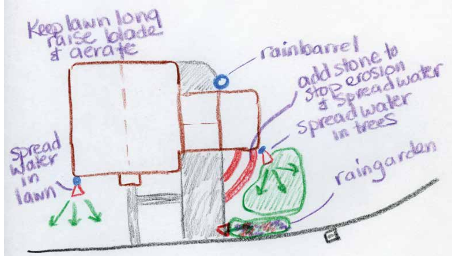
Downspout directed to lawn with end piece to spread water
