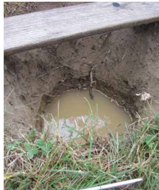
Time how long it takes for the water to drain. Repeat this to get three measurements.
