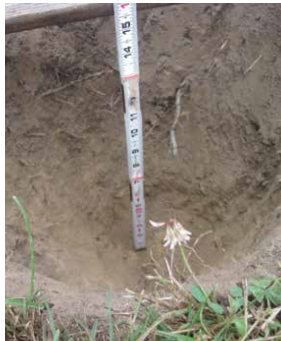
Use a ruler to measure down from the top of the water to the bottom of the hole.
